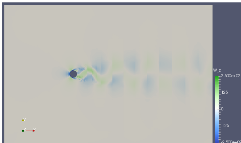
Figure 4.2 Instantaneous Vorticity Flow Field
