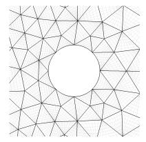
**Figure 2.1** Initial triangular mesh generated by NekMesh and visualised in VisIt, using 8 subdivisions.
